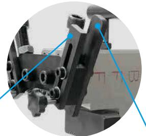
Pads at the bottom, are for tension the machine to the flange surface and protect it from falling out of the flange in case of a collision.
