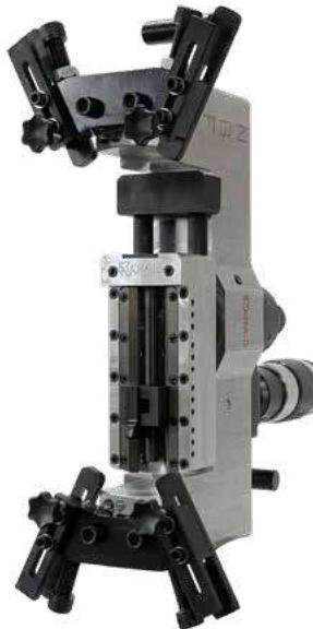
The standard locking system consists of two jaws. One of them is a stabilizing jaw with two adjustable screws to fit the outer diameter of the flange. The second jaw has three clamping screws. Both jaws are equipped with pair top pads for levelling on the sealing surface of the flange. Pads at the bottom, are for tension the machine to the flange surface. Pads help to fix the machine in any position and protect it from falling out of the flange in case of a collision.
